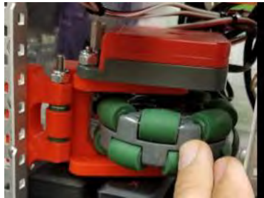
Figure 12.0: Odometry Pod V3 Mounted on Chassis
