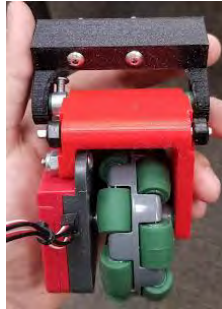
Figure 11.0: Odometry Pod V2 Assembly
