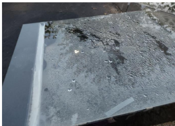
Figure 5: Evaporated water collecting on the ceiling of the still
