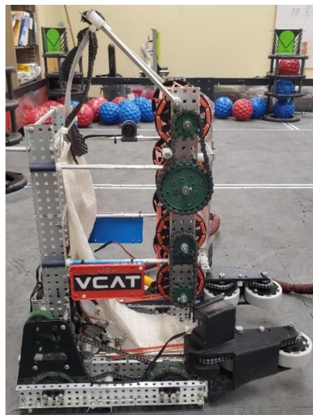
Figure 8. Side Profile of Conveyor System
