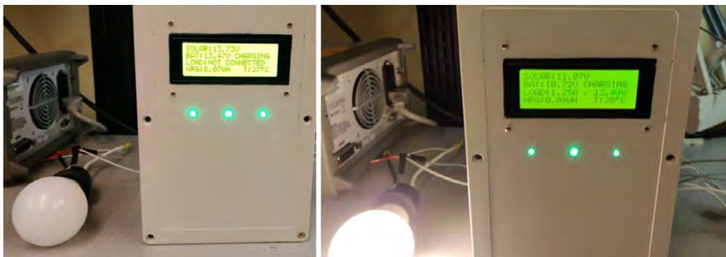
Figure 17: Solar Charge Controller LCD Display
