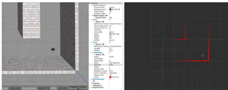
Figure 4: Gazebo(left) and RVIZ(right) Used to Visualize LIDAR Data
