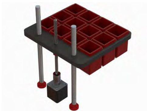
Figure 3: Z Axis Movement Mechanism
