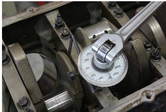
Figure 3: Angle Controlled Tightening Method [4]
