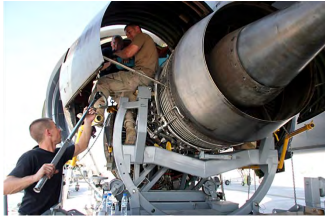
Figure 1: Technician using Torque Wrench for Engine Change [1]
