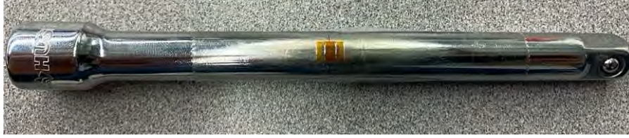
Figure 12: Torque Wrench with Strain Gage
