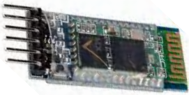
Figure 14: HC-05 Bluetooth Module
