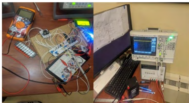
Figure 15: Testing the Charge Controller Circuit
