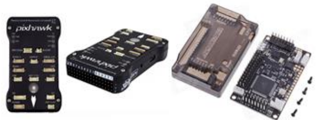
Figure 6. Flight Controllers. Pixhawk(Left), APM(Right)
