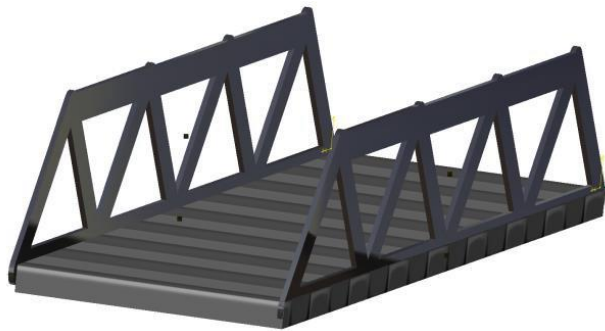
Figure 3: CATIA design of a Warren truss bridge
