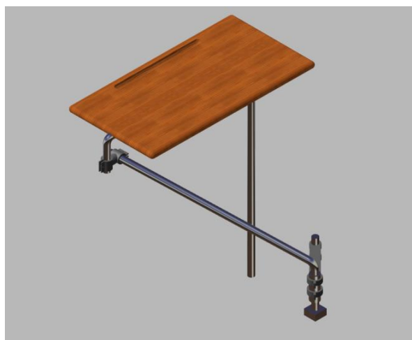
Figure 4: This is the Current Design of the tabletop model for the wheelchair
