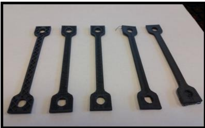
Figure 1: 20,40,60,80,100% infill from left to right
