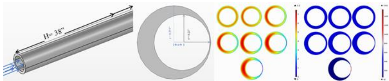
Velocity magnitude (lower left) Temperature for fully developed annular flow for different eccentricities
