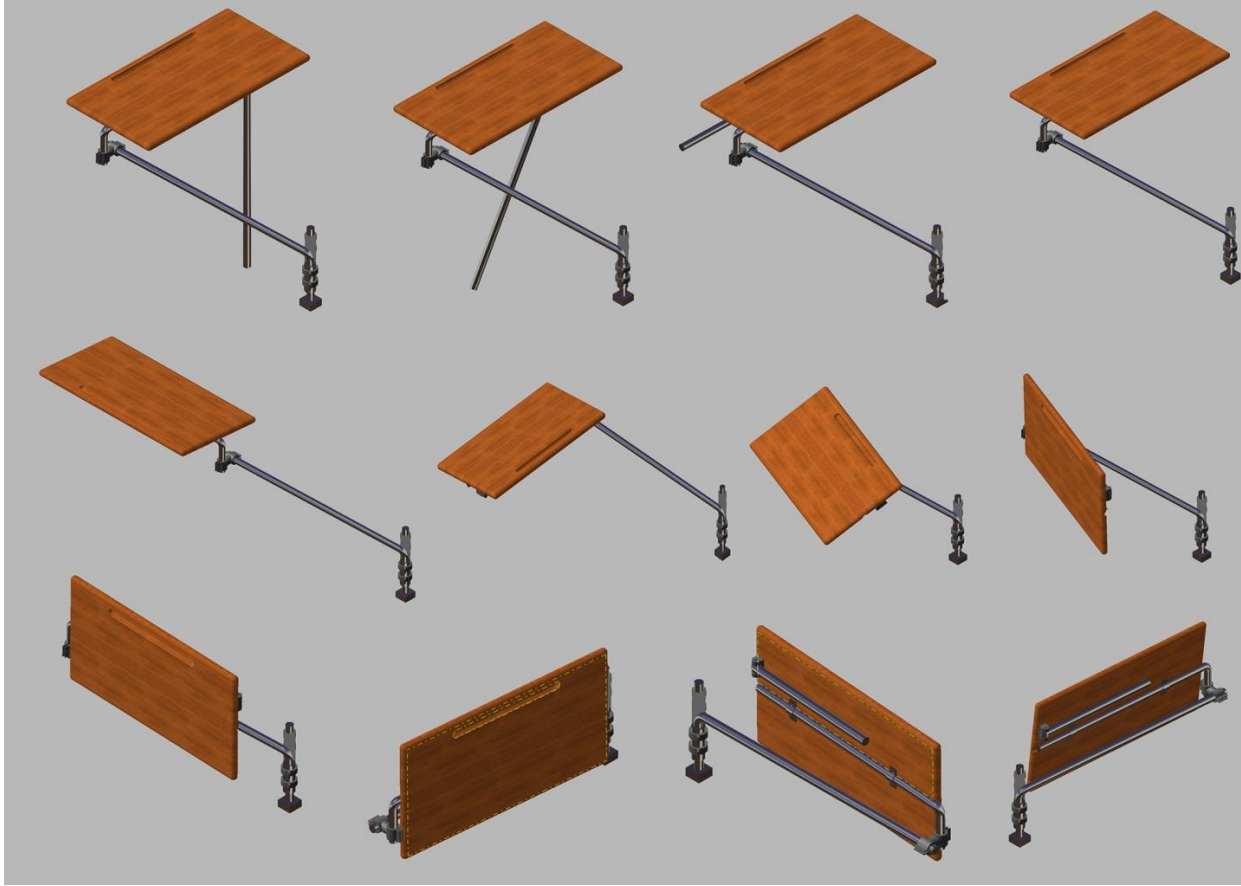
Figure 5: How the table folds: Step by Step
