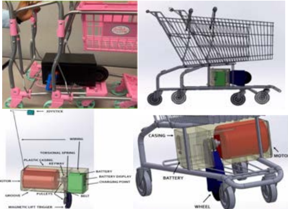
Figure 15 shows the carts stacked on prototype (top left), carts stacked on Solidworks (top right), and individual components of Solidworks rendering (bottom)
