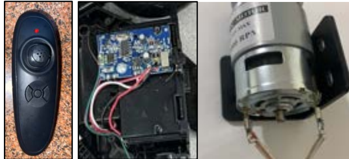
Figure 13 shows the joystick (left), speed regulator module (center), and motor (right).
